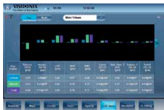
Analysis of aberrations with Zernike coefficients
