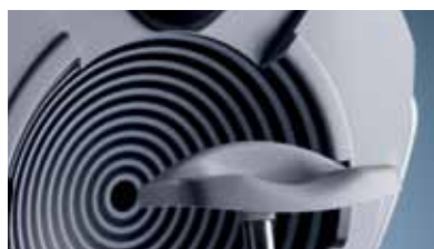
Placido disk - Measurement of corneal curvature radius
